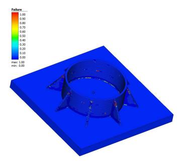
Figure 4: User-defined field of failure probability criterion, showing the vulnerable areas. Analysis method developed by Pål Idar Ingebo, Effee Induction AS.
