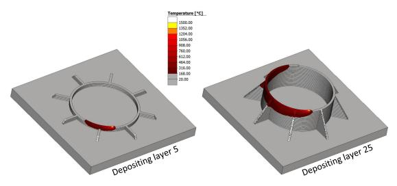
Figure 1: Temperature field comparison when the 5<sup>th</sup> layer and the 25<sup>th</sup> layer are being deposited. **Robot tool path developed by Terje Alfsen, Effee Induction AS.**
