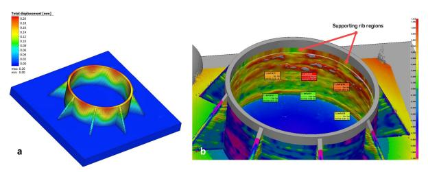
Figure 2: (a) Calculated displacement field, showing how the material is deformed under the given tool path and (b) comparison between the nominal CAD dimensions and the 3D-scanned geometry after deposition.
